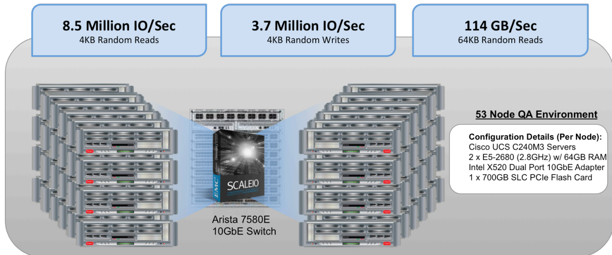
Figure 9. 53-node ScaleIO QA Environment Audited Scaling Test Results
