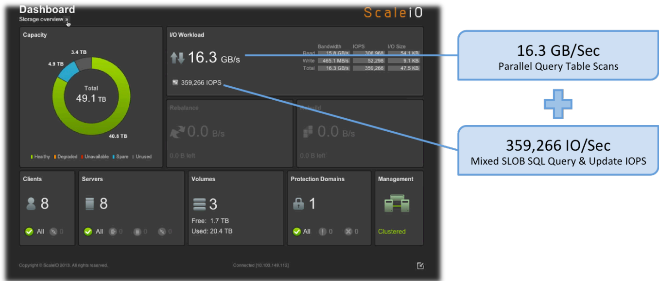
Figure 11. Eight-node Oracle RAC Environment: Oracle Parallel Queries with Simultaneous OLTP Mixed Workload
