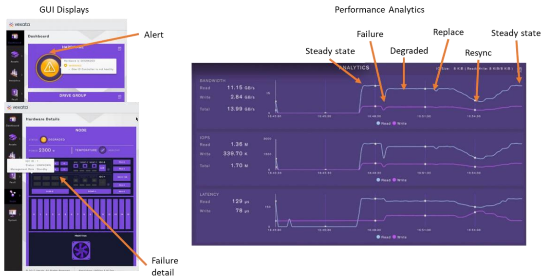
Figure 9. I/O Controller Failure and Recovery
