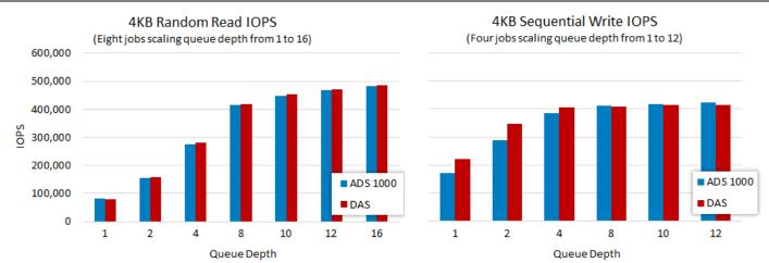
FIGURE 1. ADS1000 to DAS Comparison of NVMe SSD IOPS Performance
